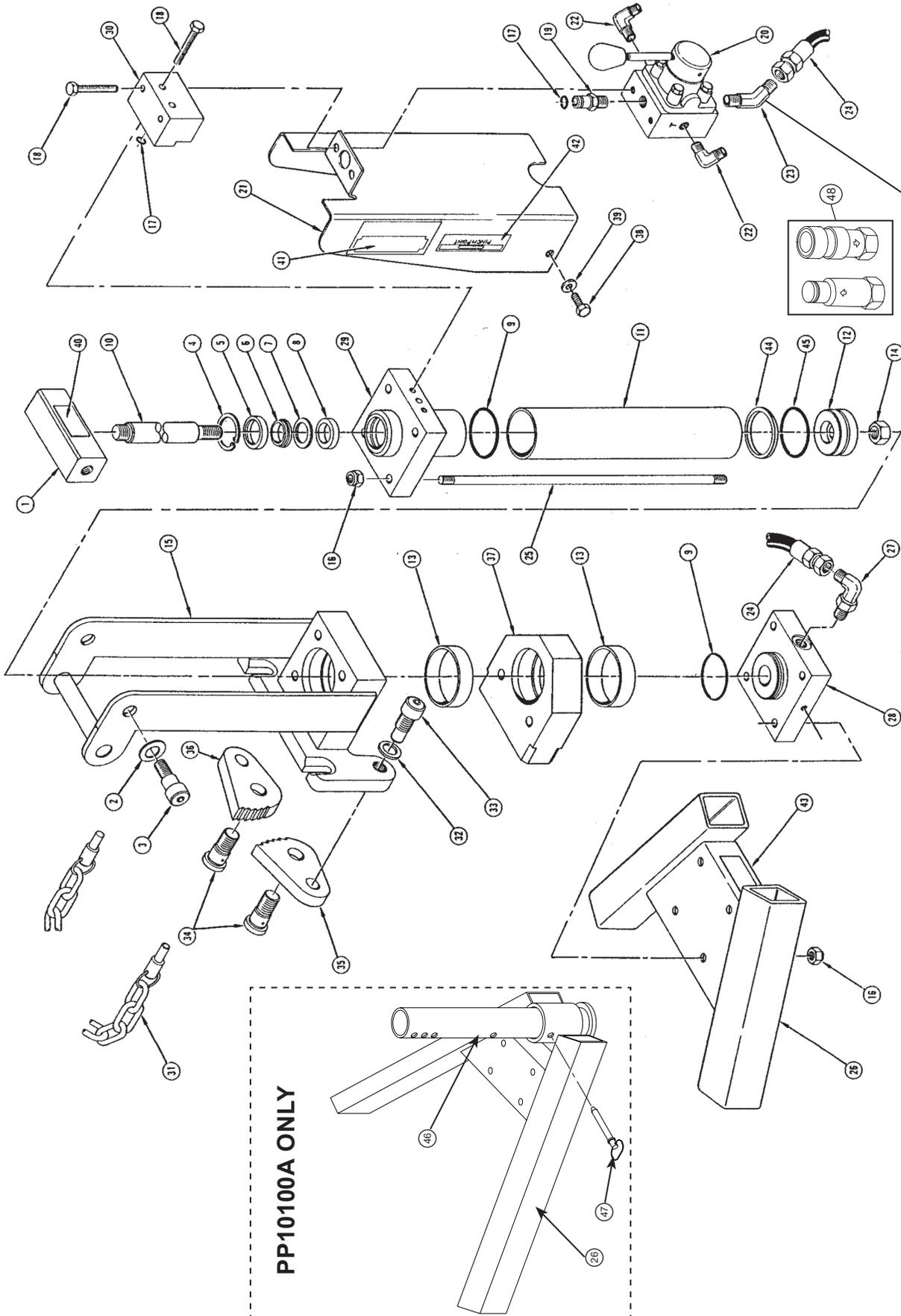
Note: Item # 23 has changed from a 45° elbow to a straight Adapter P/N-00946 in November 2011.
